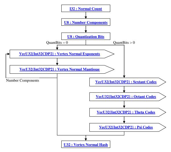
Figure 228: Compressed Vertex Normal Array data collection
