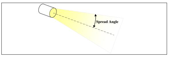
Figure 57: Spread Angle value with respect to the light cone
