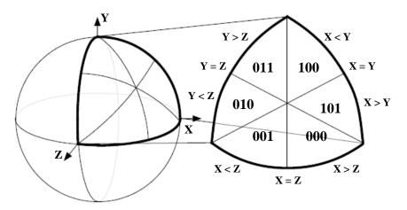
Note that the sextant three bit code assignments used by the JT format (as seen in <u>Figure 244</u>) are slightly modified from the original assignments as specified by Deering.
