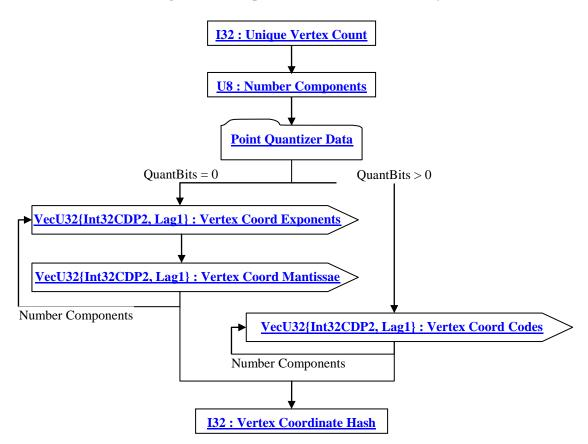
Figure 227: Compressed Vertex Coordinate Array data collection
