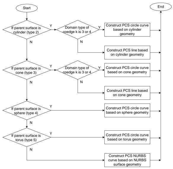
Figure 212: MCS Curve Recovery from Surface Geometry
