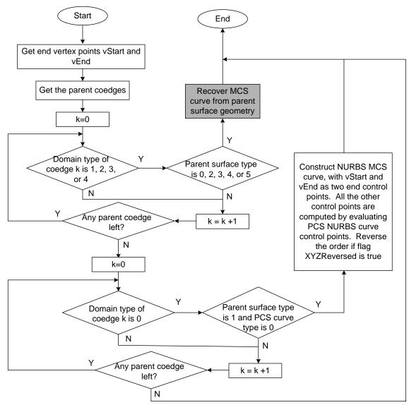
Shown in Figure 212 is the detailed description of how MCS curve can be recovered from surface geometry.
