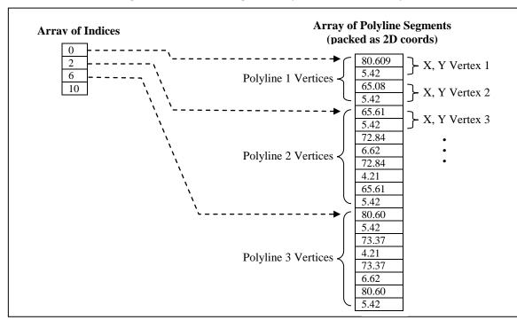
Figure 144: Constructing Text Polylines from data arrays
