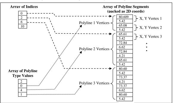
Figure 146: Constructing Non-Text Polylines from packed 2D data arrays
