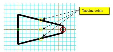
Above is a concentric reducer shown with the maximum of three tapping points.
