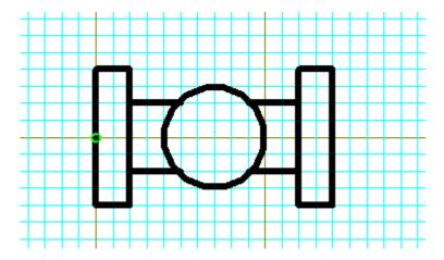
Construction of the symbol using lines & circles.
