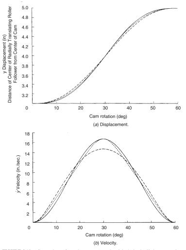
**FIGURE 3.10.** Comparison of popular curves (cam has 2-inch rise in 60-degree rotation and 3-inch pitch diameter). (Erdman and Sandor (1997) with permission by Prentice Hall, Upper Saddle River, N.J.)
