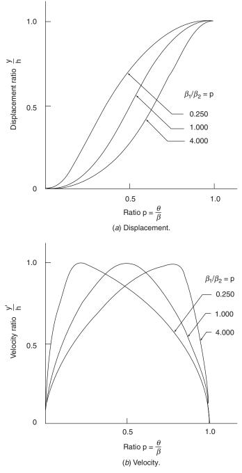
**FIGURE 3.8.** Skewed modified trapezoidal curve comparison (normalized  $h = 1, \beta = 1$ ).
