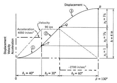
FIGURE 3.3. Example modified constant velocity curve.
