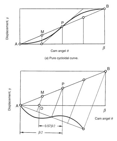
(b) Modified cycloidal curve.
