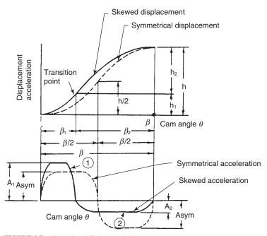
FIGURE 3.7. Skewed modified trapezoidal curve.
