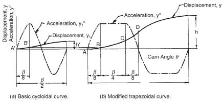
FIGURE 3.5. Modified trapezoidal acceleration curve.
