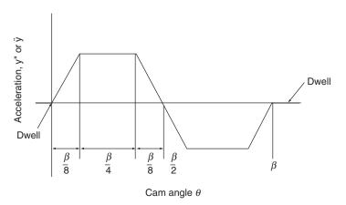
FIGURE 3.4. Trapezoidal acceleration curve-DRD cam.
